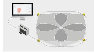
To guard large areas, up to 6 sensors can be combined in one application using a control unit. The system parameters are set using the easy-to-use confi guration software.
