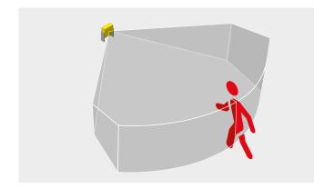
The LBK safety radar sensors detect movements and are used for guarding hazardous areas. They monitor the protected area for access by and the presence of persons. Even persons who are standing still are not really "static", and are therefore detected reliably by the sensor.
