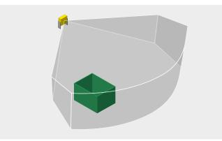
The radar technology reacts sensitively to movements. However, static objects in the monitored area do not cause the safety signal to switch off.
