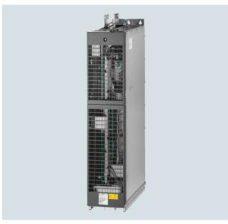
The self-commutated infeed/regenerative feedback units (with IGBTs in infeed and regenerative feedback directions) generate a regulated DC link voltage. This means that the connected Motor Modules are decoupled from the line voltage. Line voltage fluctuations within the permissible supply tolerances have no effect on the motor voltage.
