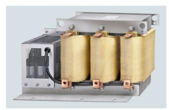
If a sine-wave filter is connected to the output of the Power Module or Motor Module, the voltage between the motor terminals is virtually sinusoidal. This reduces the voltage load on the motor windings and prevents motor noise induced by the pulse frequency.
