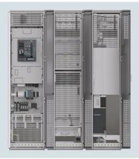
Active Line Connection Modules-2 comprise a Line Connection Module, an Active Interface Module in chassis-2 format and an Active Line Module in chassis-2 format installed in a cabinet system. They can supply motoring energy to the DC link and return regenerative energy to the line supply.
