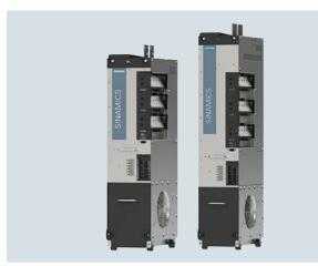
A Motor Module comprises a self-commutated inverter with IGBTs. It generates a variable voltage with variable frequency from the DC link voltage that feeds the connected motor.
