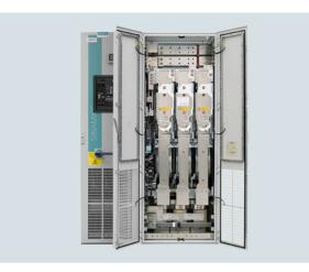
Smart Line Modules are non-regulated infeed/regenerative units. The infeed occurs over a diode jumper, while stable, line-commutated regenerative feedback takes place via IGBTs with 100 % continuous energy regeneration. An autotransformer is not required for regenerative feedback.
