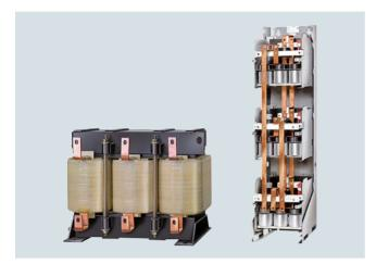
dv/dt filter plus VPL (Voltage Peak Limiter) limit the voltage rate-of-rise dv/dt to values < 500 V/ $\mu$ s and the typical voltage peaks to the following values in accordance with the limit value curve according to IEC/TS 60034-17: 2006:
