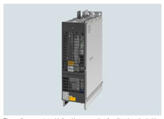
The self-commutated infeed/regenerative feedback units (with IGBTs in infeed and regenerative feedback directions) generate a regulated DC link voltage. This means that the connected Motor Modules are decoupled from the line voltage. Line voltage fluctuations within the permissible supply tolerances have no effect on the motor voltage.
