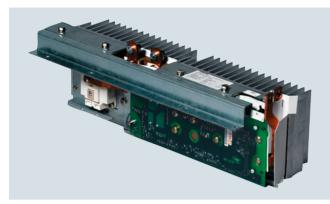
A Braking Module and the matching external braking resistor are required to bring drives to a controlled standstill in the event of a power failure (e.g. with an EMERGENCY STOP) or to limit the DC link voltage for brief periods of regenerative operation, e.g. if the Line Module is not capable of energy recovery.
