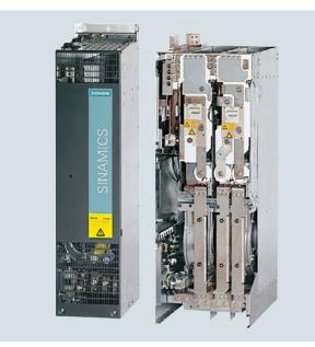
The self-commutated infeed/regenerative feedback units with IGBTs generate a regulated DC link voltage. This means that the connected Motor Modules are decoupled from the line voltage. Line voltage fluctuations within the permissible supply tolerances have no effect on the motor voltage.
