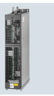
A Motor Module comprises a self-commutated inverter with IGBTs. It generates a variable voltage with variable frequency from the DC link voltage that feeds the connected motor.
