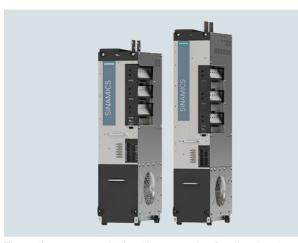
The self-commutated infeed/regenerative feedback units act as step-up converters and generate a stabilized DC link voltage that is 1.5x greater (factory setting) than the nominal voltage of the distribution system. In this way, the connected Motor Modules are decoupled from the line voltage. This improves the dynamic response and control quality because line tolerances and fluctuations do not affect the motor voltage.
