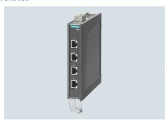
The DMC20 DRIVE-CLiQ Hub Module is used to implement a star-shaped topology of a DRIVE-CLiQ line. Two DMC20 DRIVE-CLiQ Hub Modules can be connected in series (cascaded).
