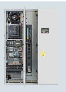
Basic Line Connection Modules are compact line infeeds for two-quadrant operation, i.e. no regenerative feedback. They are used when energy need not be fed back into the network.
