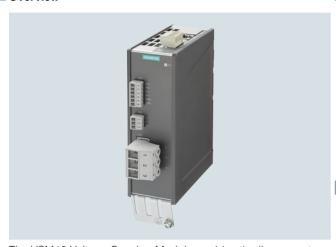
The VSM10 Voltage Sensing Module enables the line or motor voltage characteristic to be measured precisely. The phase differential voltage can be measured, either grounded (in the delivery state with jumper plugged in) or isolated.
