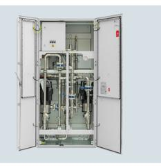
Heat Exchanger Modules are used to dissipate the power loss from the converter. They comprise a deionized water circuit on the converter side and a raw water circuit on the plant side.
