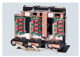
dv/dt filters compact plus VPL (**V**oltage **P**eak **L**imiter) limit the voltage rate-of-rise dv/dt to values of < 1600 V/ $\mu$ s and the typical voltage peaks to the following values in accordance with the limit value curve A according to IEC 60034-25: 2007:
