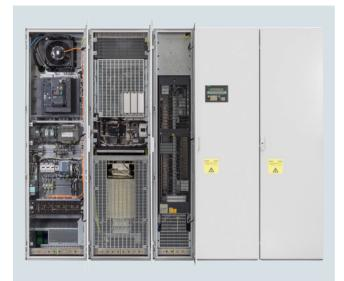
Active Line Connection Modules comprise a Line Connection Module, a liquid-cooled Active Interface Module and a liquid-cooled Active Line Module. They can supply motoring energy to the DC link and return regenerative energy to the line supply.
