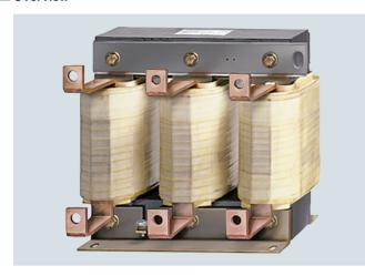
Motor reactors reduce the voltage load on the motor windings by reducing the voltage gradients at the motor terminals that occur during converter operation. At the same time, the capacitive charge/discharge currents that place an additional load on the converter output when long motor cables are used, are reduced. For group drives, output reactors should always be used. The maximum permissible output frequency when a motor reactor is used is 150 Hz.
