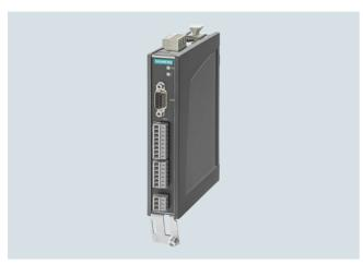
The TM41 Terminal Module supplies TTL signals which emulate an incremental encoder, e.g. to a higher-level control. The encoder interface (incremental encoder emulation) can be linked to an encoder signal from the Control Unit, e.g. incremental encoder sin/cos, by parameter assignment.
