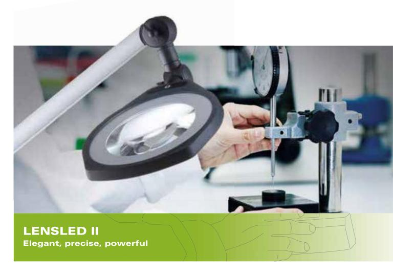
The LENSLED II is the magnifying lamp par excellence. Developed for stationary use at assembly or control workstations, the LED light with its magnifying lens can be positioned as desired thanks to the aluminium spring arm. The extremely scratch-resistant lens is made of glass and offers 1.85x magnification. The high-intensity illumination of the magnification area is free of shadows and glare, and the luminous intensity can be adjusted via infinitely variable dimming.
