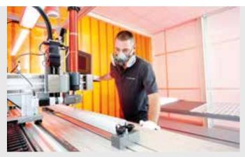
CNC-controlled glue robots
