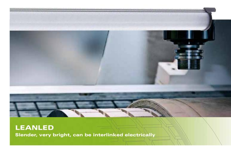
Due to its extremely compact design (25 x 30 mm), the LEANLED can be used in almost any machine space without chip bombardment or coolant (IP54). A polycarbonate cover protects the LED chips from dust and splash water. The electrical interlinking enables very simple and quick installations that can illuminate large production areas homogeneously and uniformly.
