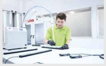
Coating machine for LED coating with PUR
