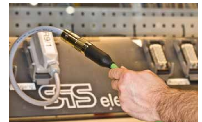
100% tested: digital continuity test
