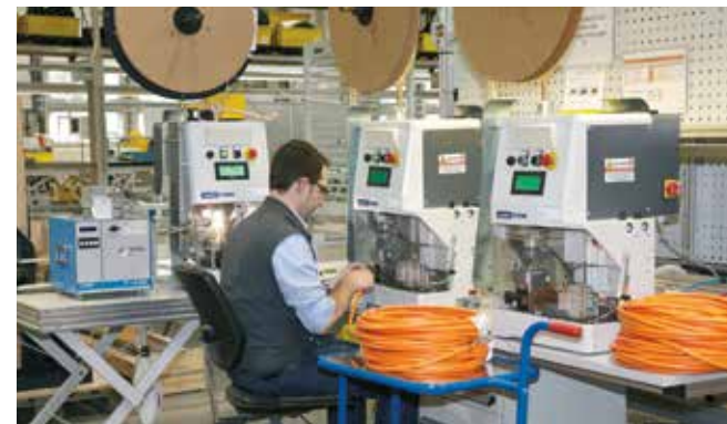
Modern machinery - automatic stripper-crimper
