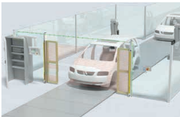
Figure 1: Process-controlled access guarding with Smart Process Gating (SPG)
